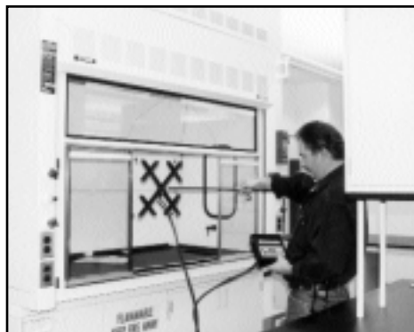
Dick Wirt (above), Paul Latus (right), are verifying critical air flows for hood exhaust and make-up air in the laboratory.
